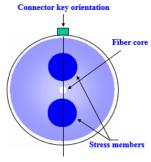
Slow axis align with connector key
